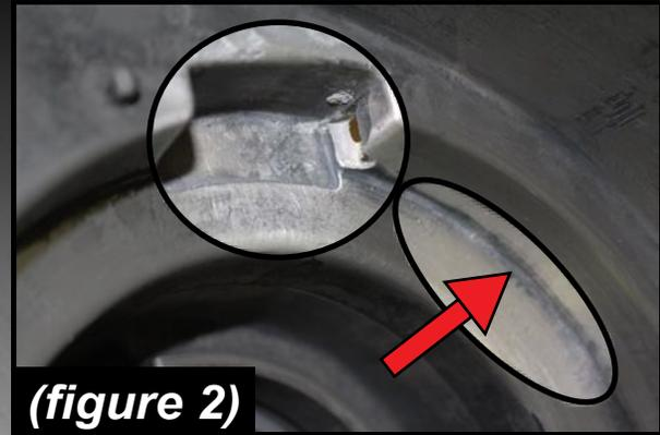
Note: Some case halves will need to be modified in this corner area so BRNY will sit flush when assembled
